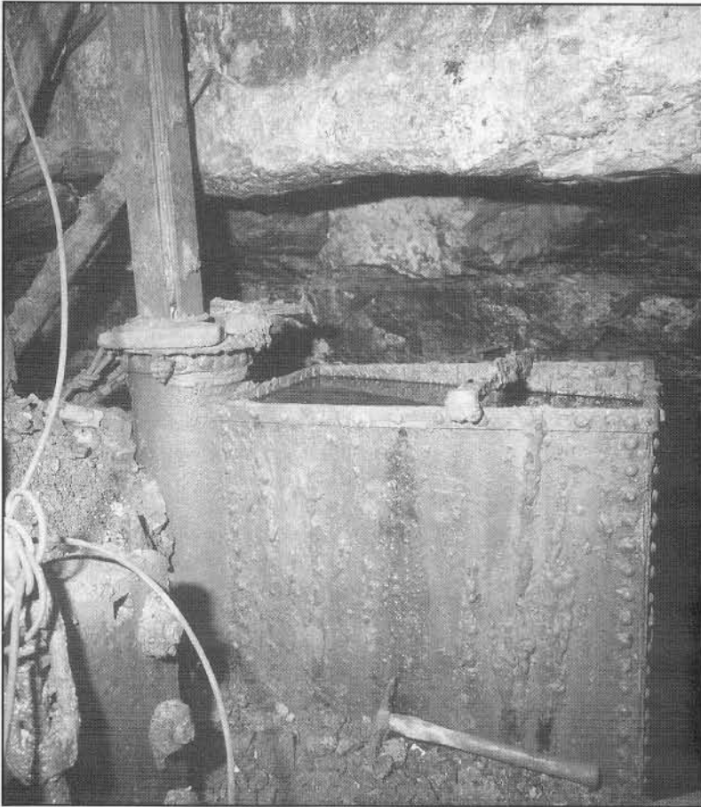
(Above) Wrought iron cistern and top of lift pump.
