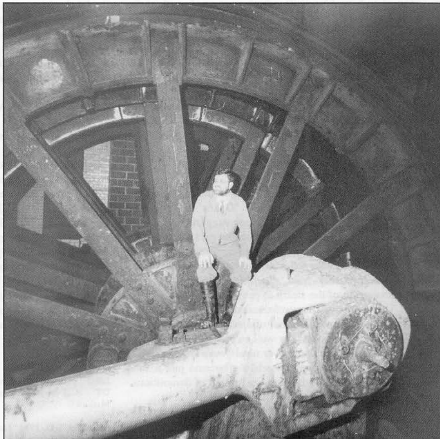
The Markham engine winding drum and crankshaft, in late 1995. The scale is Bob Metcalfe (Photo: Paul Deakin).
