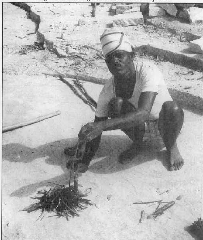
Plate 5. Small fire burning over the chisel which transmits the heat down into the granite making the incipient crack spread.
