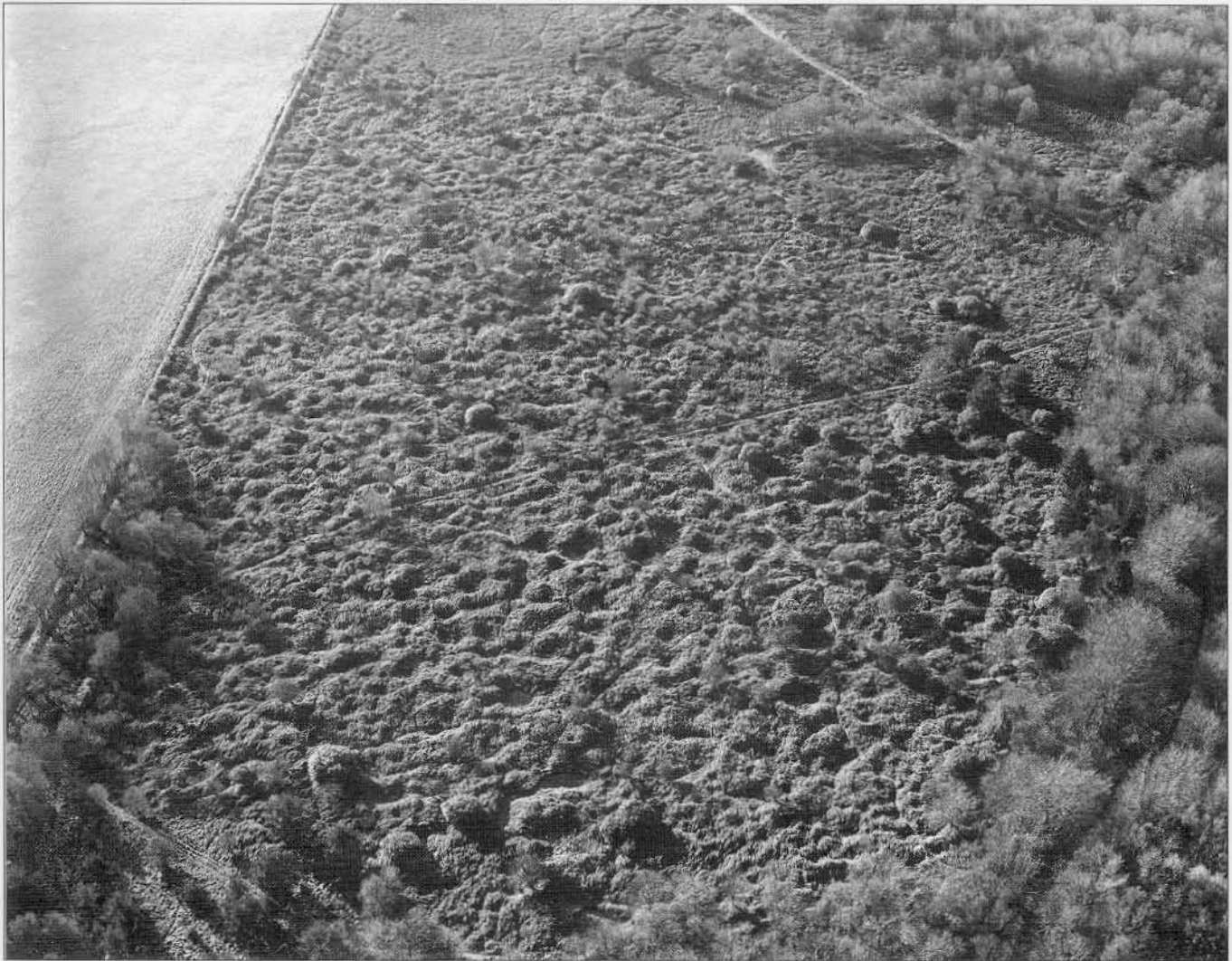
Plate 3. Aerial view of the iron extraction pits at North Hill Common. The abrupt change at the boundary line in the top left-hand corner represents the limit of reclamation, the pits originally continued well beyond this line (F.M. Griffith DCC, 1993).
