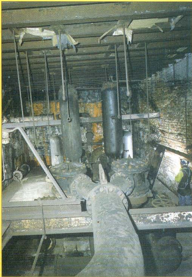
Mining for water: Manton Colliery, near Worksop: (top) Pumping chamber with late 19th century Joseph Evans' pumps., replaced by (right and below, left) ram pumps c.1940 and, in turn, (below right) c.1960 electrically driven centrifugal pump. (Photos: Paul Deakin).
