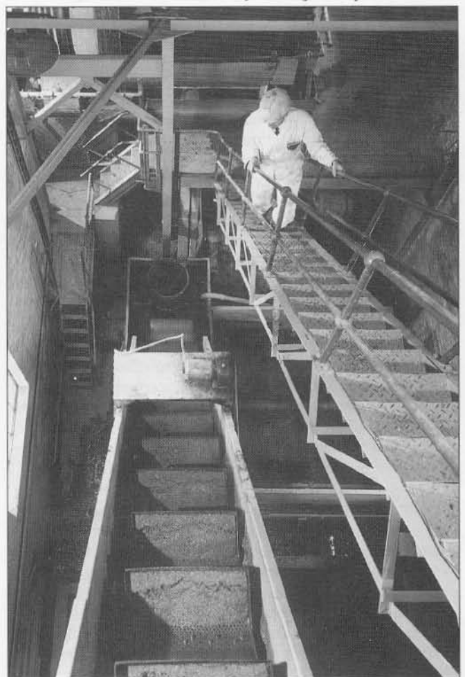
Cavendish Mill. Bucket elevator on left. The mill was visited by members of the 1997 NAMHO Conference (photo by H.M. Parker.
