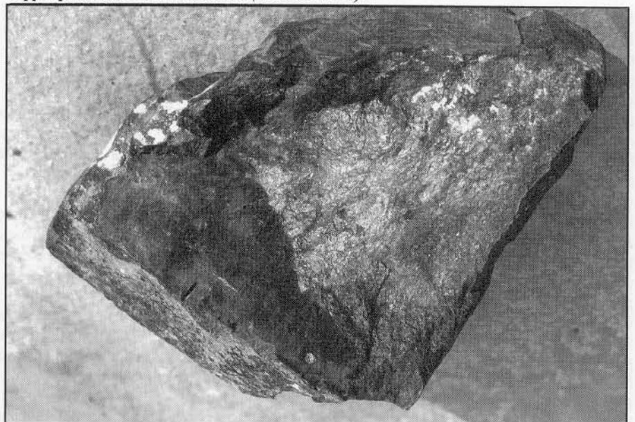
Plate 1. Slag sample A, Beaumaris (4/9/1993), showing fresh brick with iridescence and copper prills. Size 14 x 10 x 10 cm. (Photo: NVCB.)
