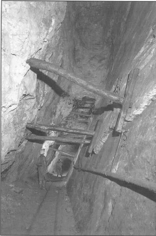
Plate 1. Inclined open stope in Long Rake which had a full width of calcite, and with a rib remaining on the right-hand wall. (Photo - Paul Deakin).
