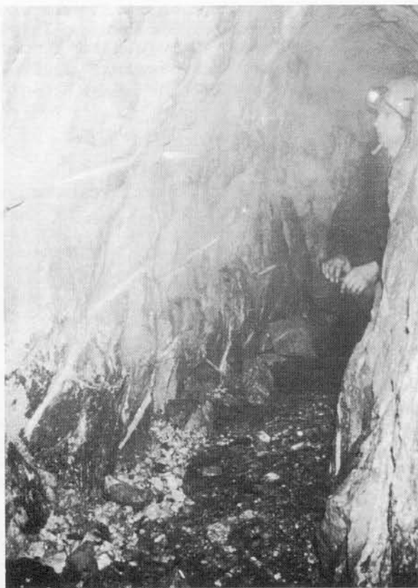
4. Shot-holes in the Greatorex-Bedehouse branch level - probably the earliest mining shot-holes still accessible in Britain.
